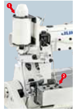
1 Presser lifter drive mechanism 2 Thread trimmer drive mechanism
